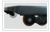
Additional entry rollers ensure easy pallet entry and preventing possible damages.
