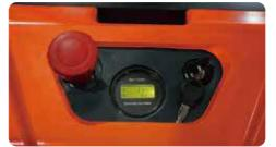
Battery deep discharge protection device, voltage discharge indicator with low voltage automatic cutting and lifting function, for higher battery lifetime. Proofed emergency switch and voltage discharge indicator, make it more durable and reliable.
