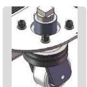
Convenient stability casters adjustment, no need for lifting the stacker.
